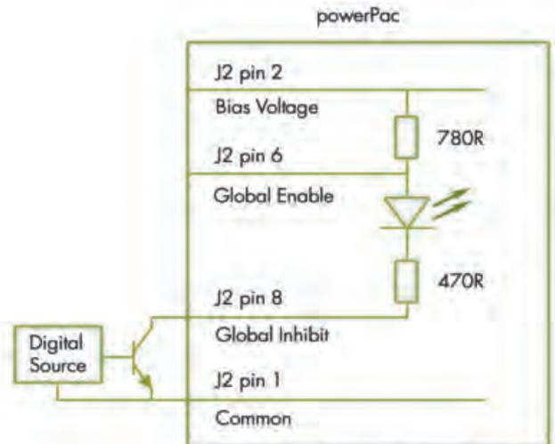
Global Inhibit Using an External Signal
