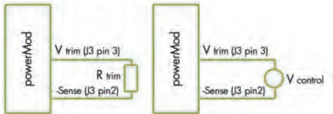
Remote Output Voltage Adjustment of powerMods
