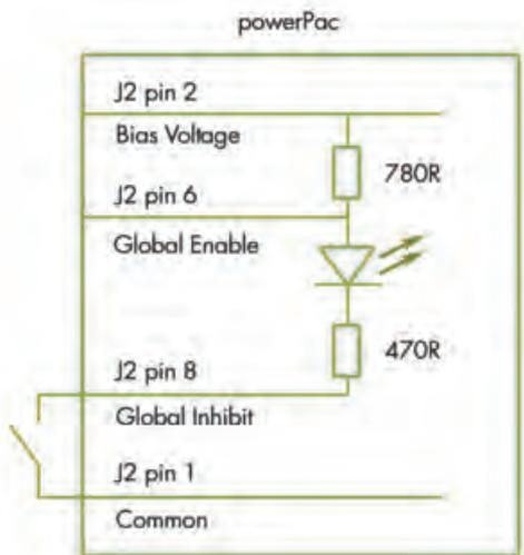
Global Inhibit Using Bias Supply Voltage
