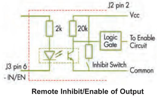
**Remote Inhibit/Enable of Output**
