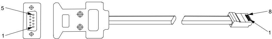
Fig. 5-7: RS485 cable with DB-9 connector.
