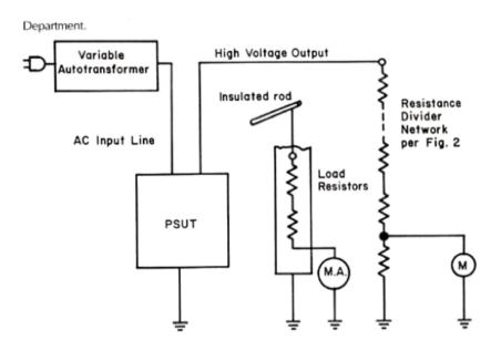
Variable Autotransformer - 105-125V AC, 50/60 Hz, Wattage as required to supply PSUT.
