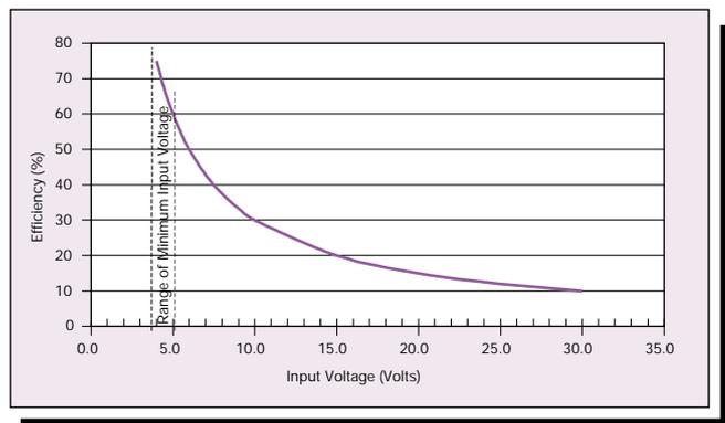
Figure 1.2 - Maximum Efficiency of 3V Linear Regulator
