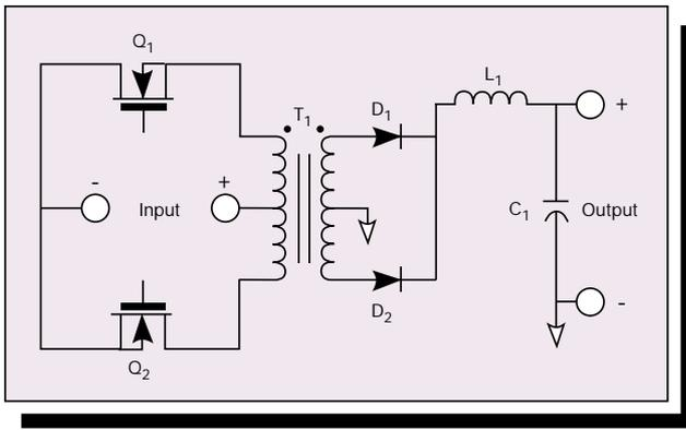
Figure 1.12 - Push-Pull Converter
