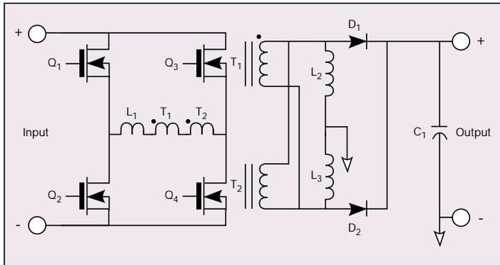
Figure 1.15 - Phase Shifted Full Bridge Converter
