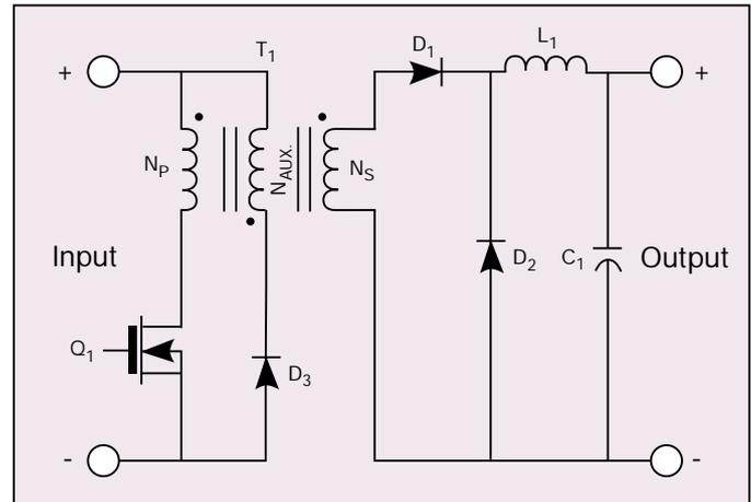
Figure 1.9 - Forward Converter
