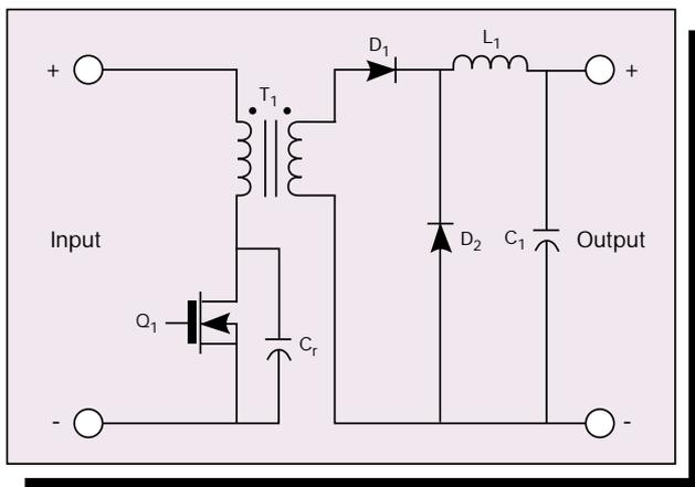
Figure 1.10 - Resonant Reset Forward Converter
