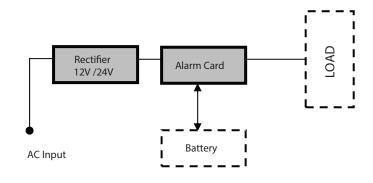
Fig 1: Block Diagram.
